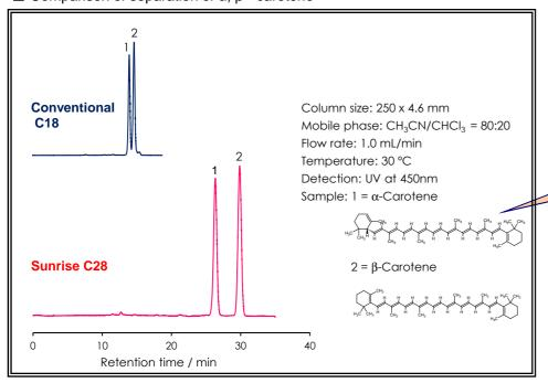
The mobile phase including chroloform makes alkyl chains brash up because chroloform can enter among alkyl chains. Consequently retention times of C28 became 2 times longer than C18.
