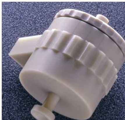
HF-resistant spray chamber, used in conjunction with ceramic sample tube and V-groove nebulizer provides a glass-free sample path for silica-based samples
