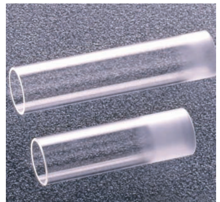
Extended outer tube for the Integra torch, shown here with standard glassware
