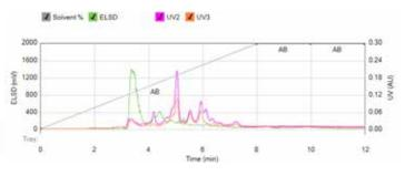
Purification of Neem Oil, 500mg on a REVELERIS<sup>®</sup> 40g silica cartridge (upper) and a REVELERIS<sup>®</sup> HP 40g silica cartridge (lower).
